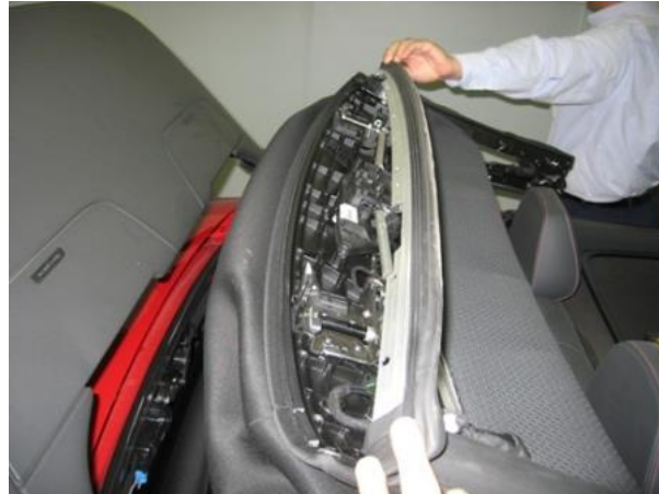
Figure 5. Retaining strip and seal pulled back.
