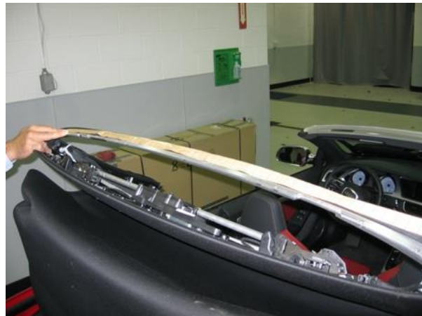
Figure 6. Butyl cord application.
