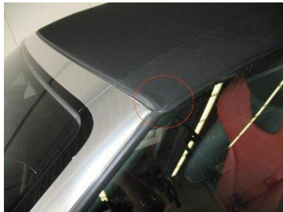
Figure 1. Location where a leak may occur.
