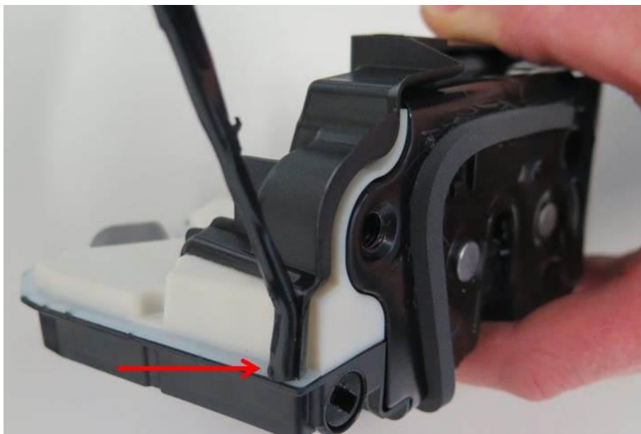
Figure 3) starting position for routing Butyl sealing cord
