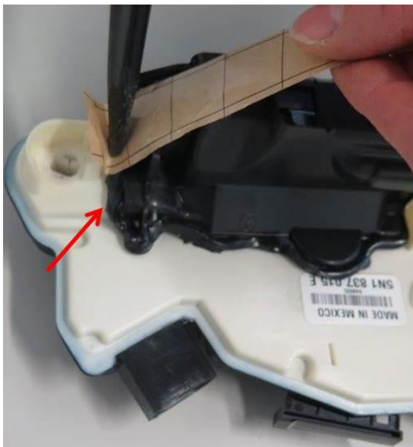
Figure 5: pressing down Butyl sealing cord with suitable tool
