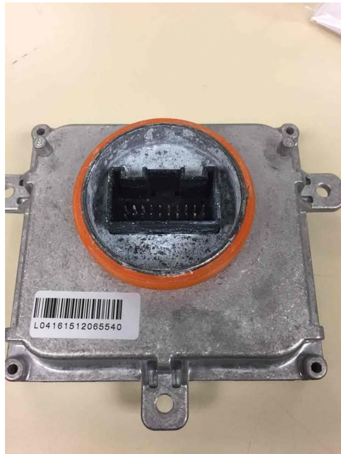
Figure 1. LED control module with evidence of water ingress.
