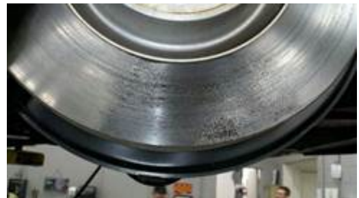
Figure 4. Corrosion marks on the brake disc.
