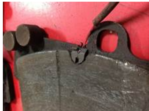
Figure 6. Worn brake pad.
