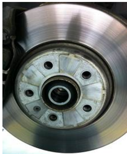
Figure 7: Brake disc with heat marks.
