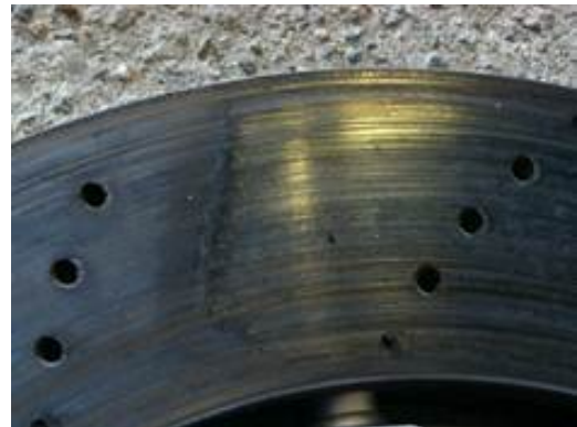
Figure 5. Deposits on the brake disc.
