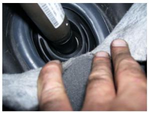
Figure 1. Sealing sleeve on the bulkhead.
