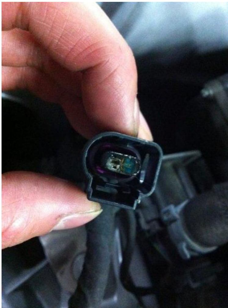
Figure 2. Corrosion formation on the connector pins.
