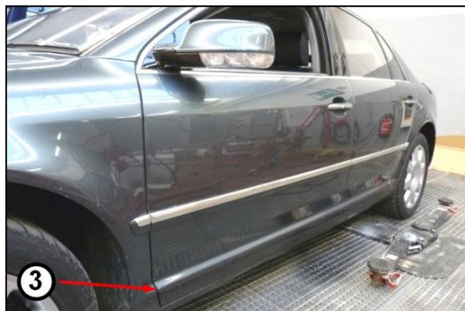
Figure 3 – Lower protective strip
