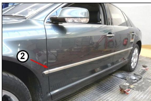
Figure 2 – Central protective strip
