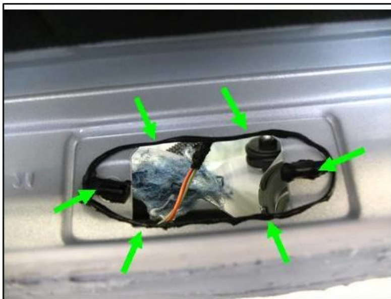
Figure 3) License plate light, contact surface and hole sealed with butyl sealing cord
