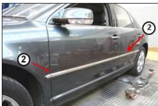
Figure 2 – Central protective strip
