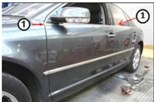
Figure 1 – Upper window channel strip
