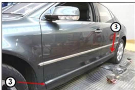
Figure 3 – Lower protective strip
