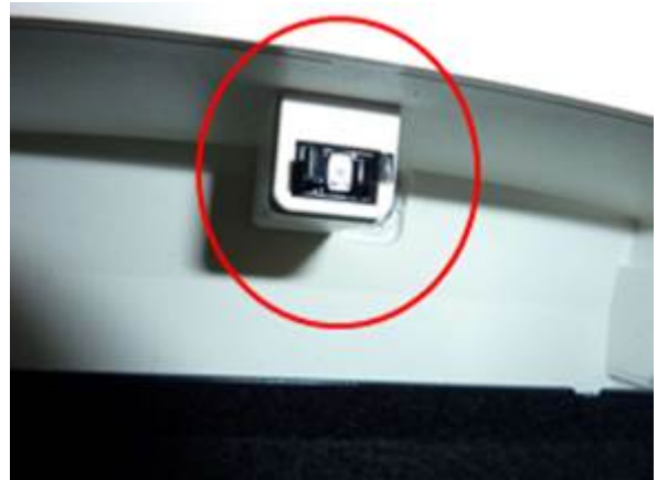
Figure 1: The sunglass holder spring latch mechanism.
