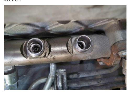
3. Install the new mounting bracket (2) (P/N: A4720701140) and two new mounting bracket bolts (4) (P/N: N910105006023) to the fuel rail clamp. Torque to 15 N·m (132 lb·in.).
