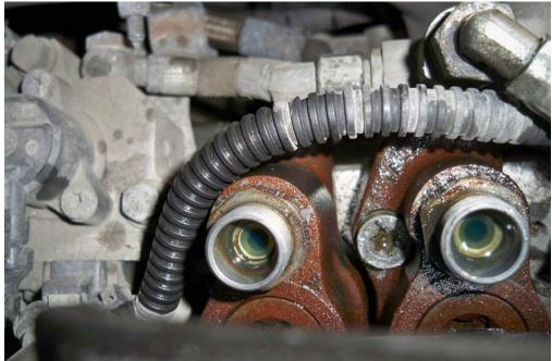
2. Clean the sealing area inside the high pressure fuel rail using a clean lint-free cloth.
