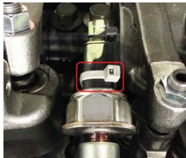
Cable tie location
