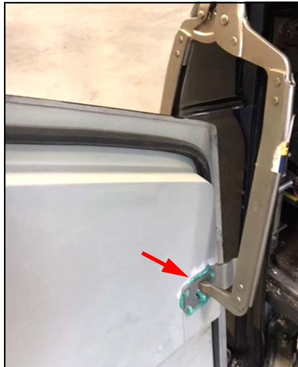
Figure 2. Bracket stopper mounting to interior face of door.
