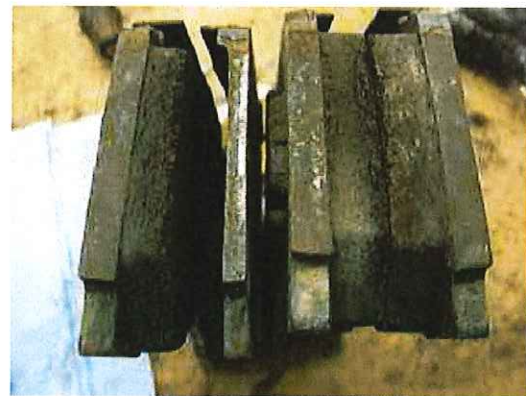
Fig. 2: showing excessive wear of outer brake pad
