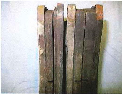
Fig. 1: showing excessive wear of outer brake pad
