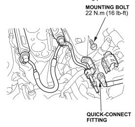
37. Remove the EGR pipe mounting bolts, then remove the EGR pipe.
