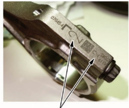
These are manufacturing marks, and do not indicate the cylinder number.
