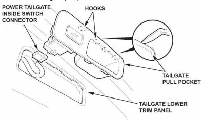
4. Pull out the tailgate lower trim panel by hand to detach the clips, then remove it.
