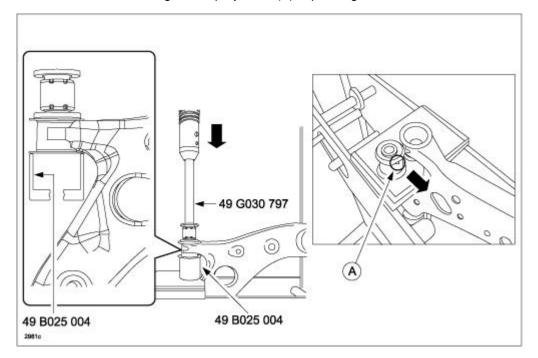
**CAUTION:** Make sure the bushing has been properly inserted by verifying that the bushing tab **IS FULLY EXPANDED**, as shown in the illustration to the left (A). The illustration to the right (B) shows an example of a bushing tab that **IS NOT FULLY EXPANDED**.
