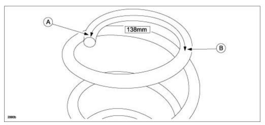
7. Install the protector (A) onto the coil spring aligning the end (slant cut side) with the marking at spot (B).
