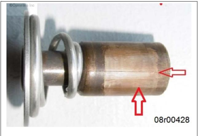
Figure 1, Coolant Thermostat with Scuffing and Cracks.
