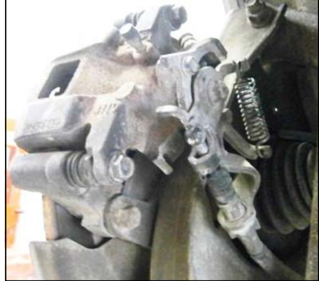
NG Condition: Parking Brake Lever Stuck
