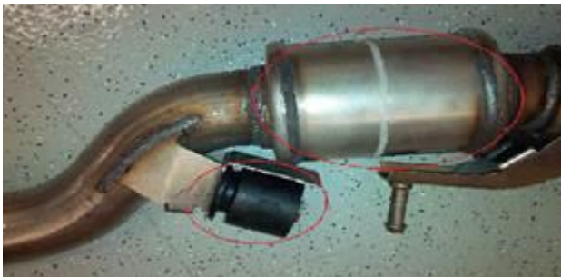
Figure 1. Dampening weight and shipping sleeve on decoupling element.
