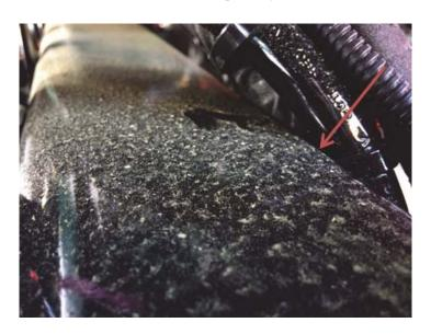
The harness should not contact the <u>edge</u> of the frame rail. If there is contact with the edge, the harness needs to be properly secured to its clipping brackets so it is able to clear the rail.
