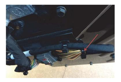
If the cable tie is found to be cutting into the wire insulation, remove the cable tie, wrap the exposed wires in harness tape and re-clip the harness securely.
