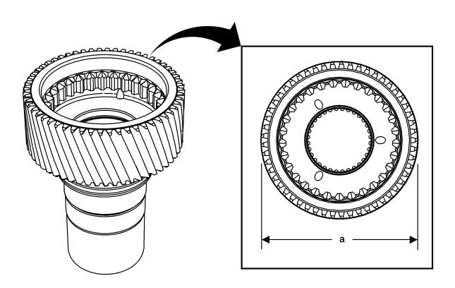
The first design input shaft can be identified as a 56 tooth design with an outside diameter (a) of 91.4 mm (3.60 in).
