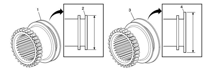
Interim 2012 model year the High/Low shift fork, fork pad and High/Low clutch design changed. The first design high/low clutch (1) can be identified by having a 73 mm (2.87 in) OD rear flange (2). The second design high/low clutch (3) can be identified by having a 76 mm (2.99 in) OD rear flange (4).
