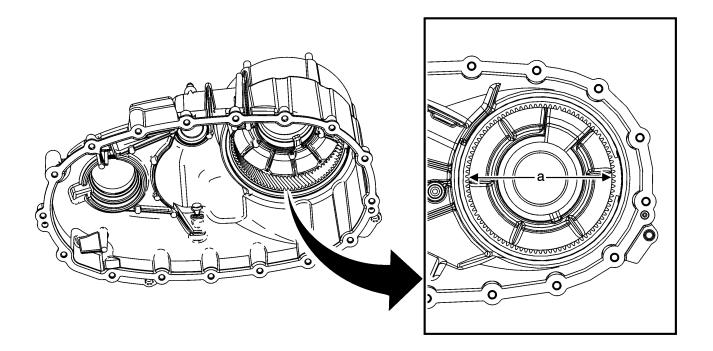
The first design front case half assembly can be identified as having an internal gear that is a 94 tooth design with an inside diameter (a) of 148.5 mm (5.85 in). The second design front case half assembly can be identified as having an internal gear that is a 91 tooth design with an inside diameter (a) of 142 mm (5.59 in).
