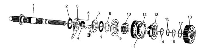
Light Duty (LD) 2007-2010 MP3023-NQH and 2010 MP3010-NP0 production transfer cases are built with LD control actuator levers (3 and 6) and are used with 13 mm (0.52 in) diameter control actuator lever balls (5).
