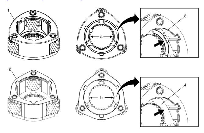
The first-design light-duty 3-pinion high/low planetary carrier (1) can be identified as having a 30 tooth design with an inside diameter (a) of 61.3 mm (2.41 in). Ir addition, the first-design carrier can also be identified by the presence of a recessed washer pocket (3) at the rear thrust washer location.
