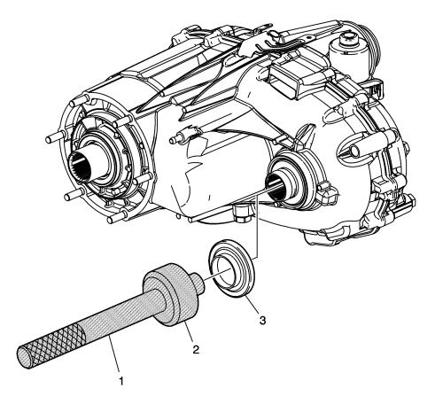
Interim 2012 model year, a new design front output shaft deflector (3) was implemented into production for second design NQF–HD/SHD and NQG–HD applications. First design 2011 model year NQF and NQG applications can be identified as not having the deflector on the front output shaft.
