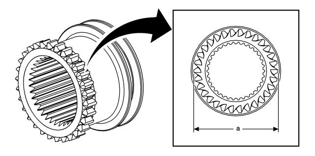
The first design high/low clutch can be identified as having a 30 tooth design with a gear tooth outside diameter (a) of 65.50 mm (2.58 in).
