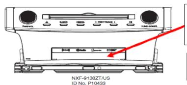
The SD card is behind this flip cover. The Micro SD needs to be removed when returning the Main Unit to Pioneer.
