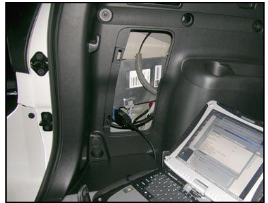
Figure 10. Diagnostic Cable Connected
