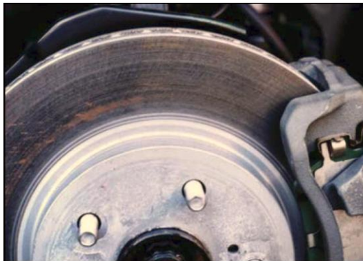
Figure 1. Slight Rust on Rotor (Easy to Remove by Braking)
