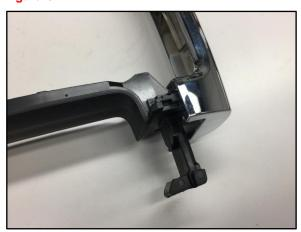
B. Seat the cover by rotating in the direction indicated by the arrow as shown.
