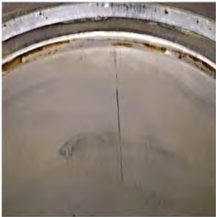
Examples of bore discoloration
