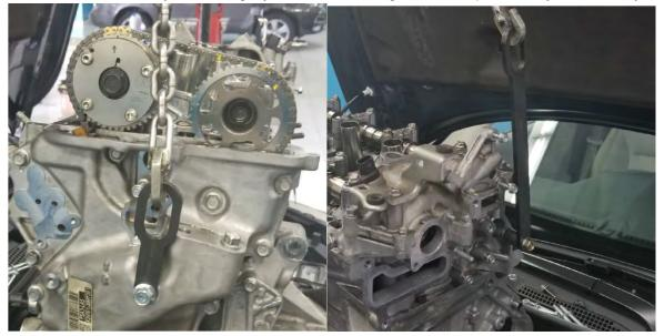
28. Secure the engine with a chain, load leveler, and engine hoist.
