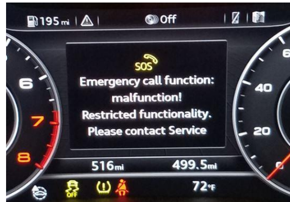
Figure 1. Warning message "Emergency call function: malfunction!"
