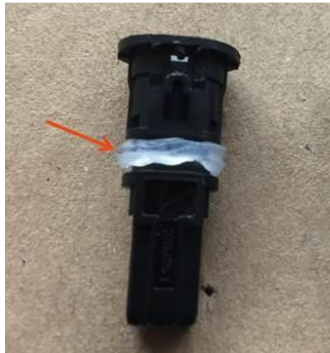
Figure 1. Damaged seal in wiring harness connector.
