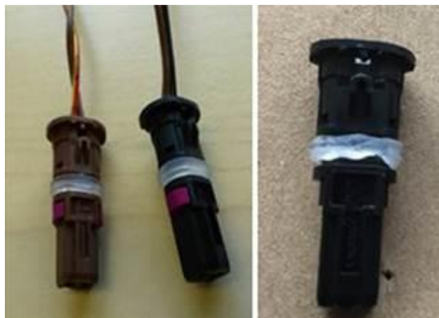
Figure 2. Damaged or white seal connector.
