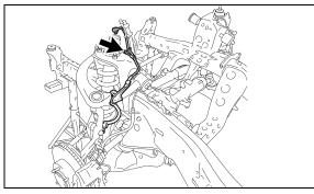
e) Remove the engine and transmission assy.
