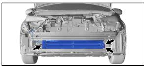
D. Disengage the two guides and remove the radiator shutter sub-assembly.
