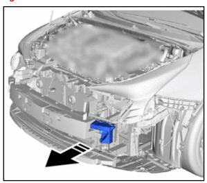
3. Remove the front bumper energy absorber as shown.
