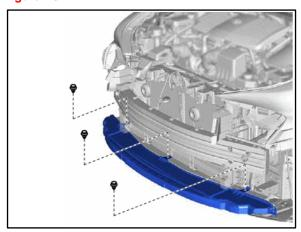
14. Install the front bumper energy absorber as shown.
