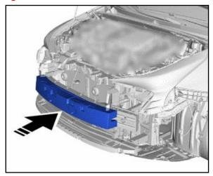
15. Install the LH and RH front energy absorber mounting reinforcement. LH installation is as shown.
