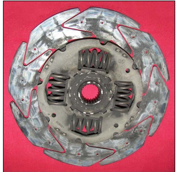
Figure 1. Clutch Disk Missing Friction Material
