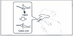
c) Insert the cable end into the inside handle as shown in the figure.
