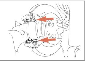
3. Remove the rear disc brake cylinder mounting.
