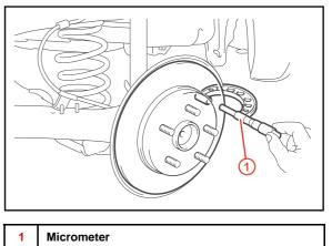
C. If the disc thickness is less than specified, replace the rear disc.
