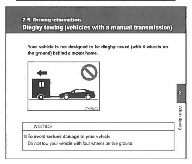
The Scion FRS is not designed to be dingly towed with all four wheels on the ground behind a vehicle. Doing so may cause serious damage to the vehicle.
