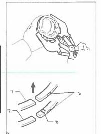
NOTE: Install the No. 2 compression ring with the code mark facing upward.
