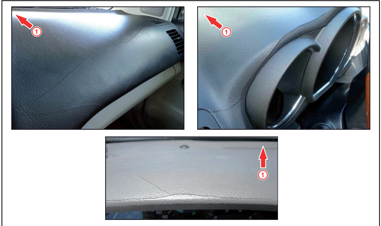
Figure 3. Examples of Cracked Condition
