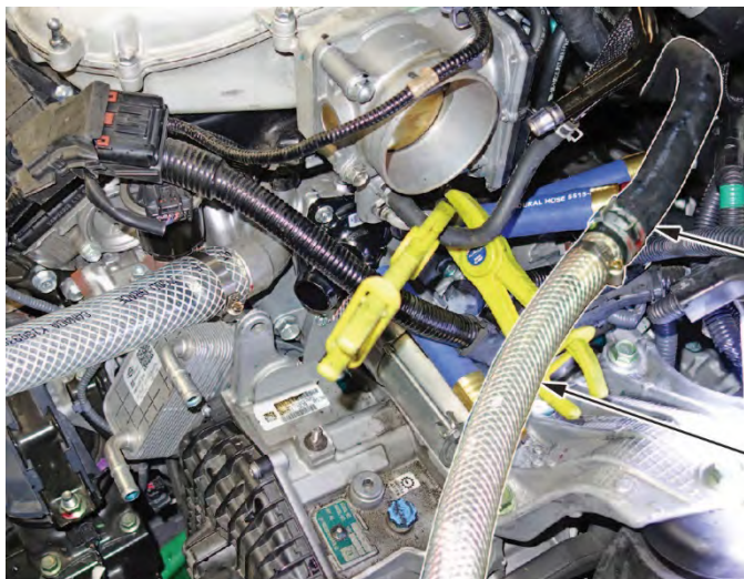
HEATER HOSE PUMP OUTLET HOSE
