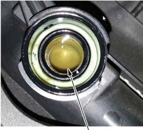
ATF IN THE COOLING SYSTEM
