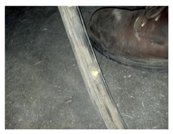
**Note:** A vehicle will sometimes show evidence of dirt/dust being pulled past the backside of the rocker moldings as shown above. A double sided tape is added to the moldings to help eliminate this condition.
