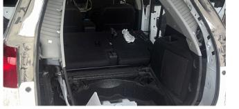
The cause of this condition may be that the dust/debris is working past the side door or liftgate sealing surfaces.
