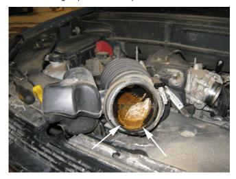
Technicians may find DTC s P0101, P0171, P0172, P0174, P0175, P1516, P2177, P2178, P2179, P2180, P2187, P2188, P2189 and/or P2190 along with eithe ice or oil deposits in the air inlet duct.
