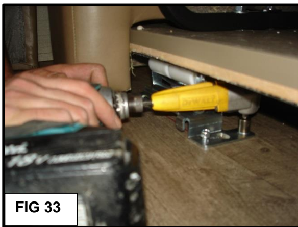
FIG 33: Install the other 3 screws on the right bracket from the front of the couch.
