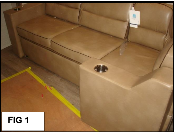
FIG 1: Rollers are under the left and right end of the sofa. Access to both corners of the sofa is required to install the rollers. FIG 2: Open the sofa seat cushion slightly to remove the kick panel from the front of the sofa. Pull straight up on the panel and the panel will come off the sofa frame. Brackets just slide over the tubular frame.
