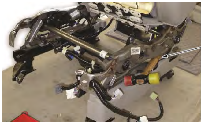
Prop open the gap between the upper and lower frame sections.
