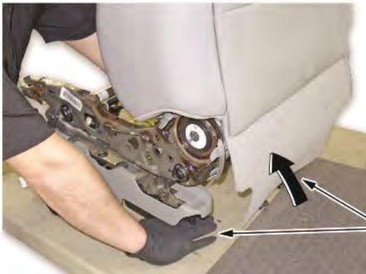
Pull upward while holding the base down.
