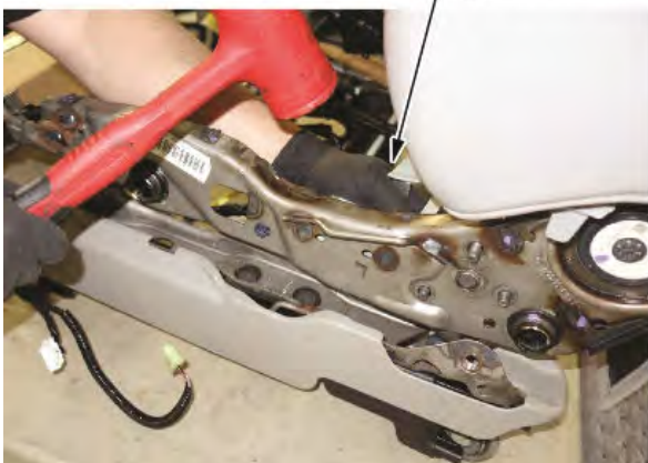
Press the VTA unit against the frame.
