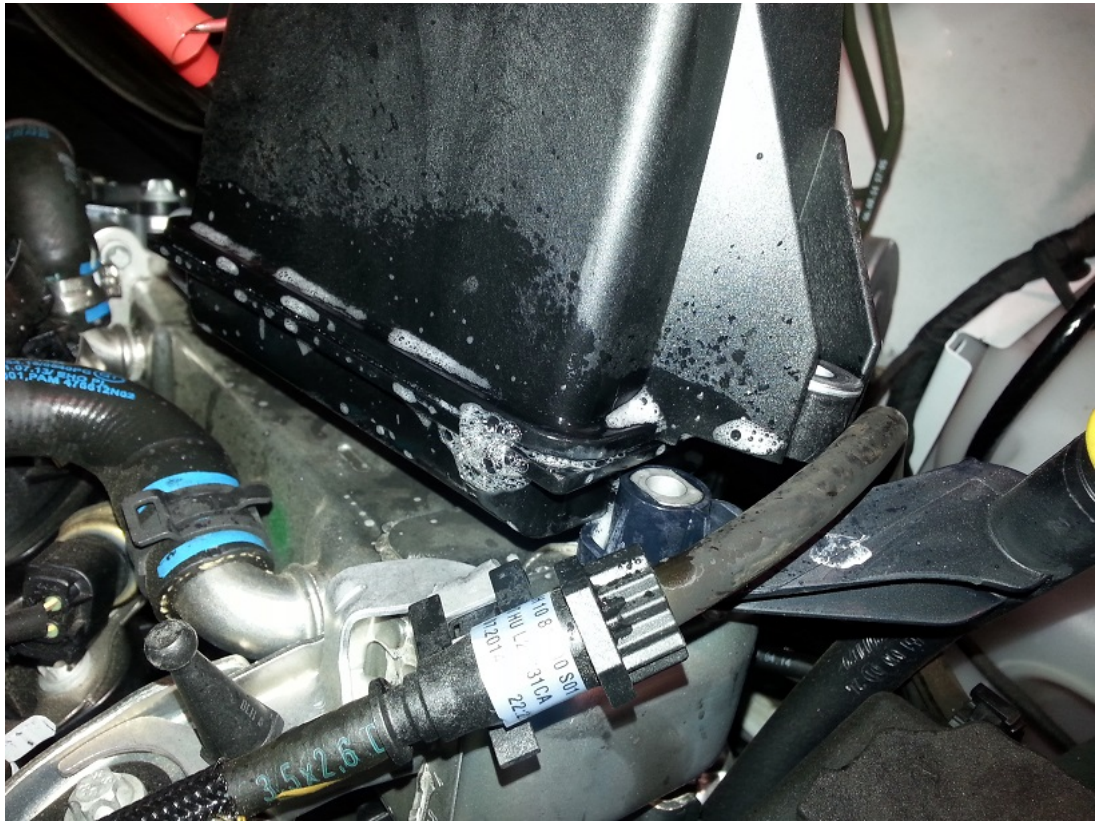
Leaking vaccum manifold.jpg:
