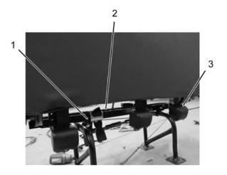
Figure 1. Main Mounting Bar.
