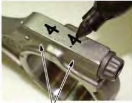
Mark the connecting rod and rod cap with the cylinder number.
