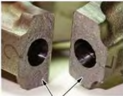
The uneven mating surfaces are uniquely matched and not interchangeable.
