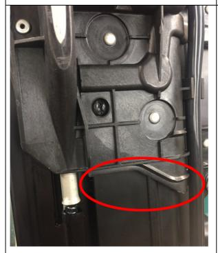
4. Using butyl rope (BMW part # 83 19 0 429 524), form into the desired shape by hand and press firmly (where indicated by circled area) onto the bottom side of the panorama unit.
