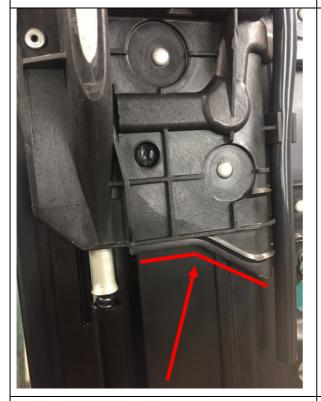
2. If the water is leaking in this area (junction between aluminum and plastic end frame of the sunroof cassette), remove all water from cassette and prepare to perform repair.
