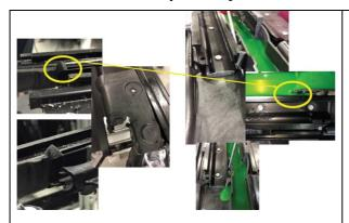
1. Refer to Repair instructions "REP 54 10 260 Removing and installing panorama glass roof". With headliner removed, identify the affected area and water test to confirm leak location.
